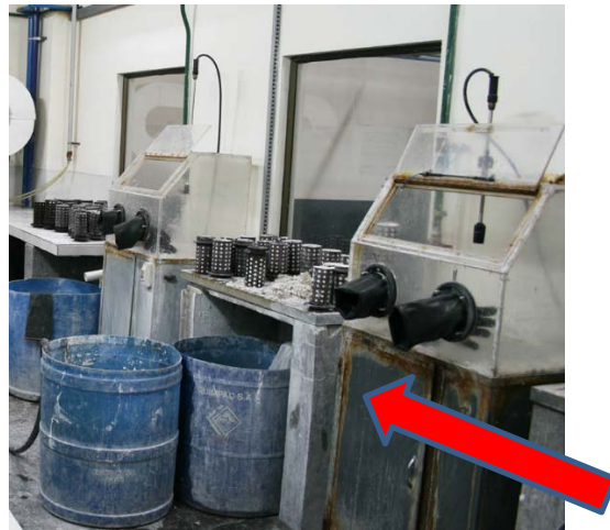
Illustration 4A: Quenching and Devesting: What not to do
