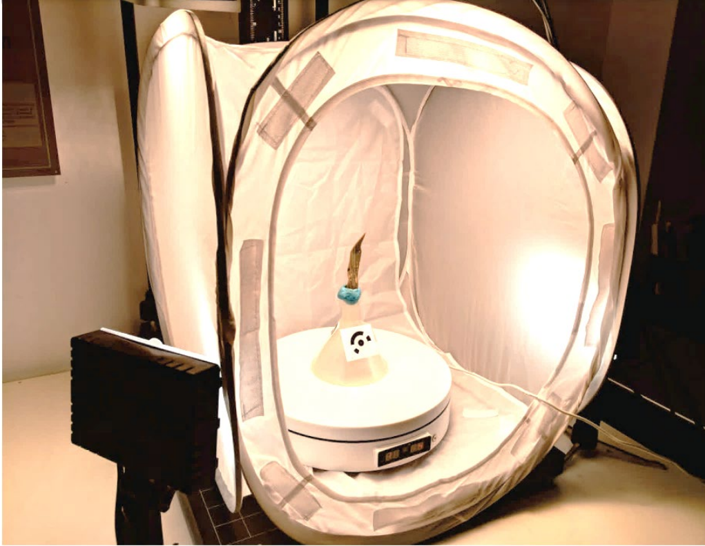
Figure 5.5: This image depicts the preparation of an artifact for photography on a turntable within a photography light box. Here, a partially ridged blade sits atop a funnel with printed identifier codes attached to aid in later model construction. The artifact is photographed from one angle, then will be adjusted so the opposite end will be in view of the camera for a second angle. The turntable stops automatically at 15-degree intervals to allow for photos to be taken. The white background aids in masking during the model production stage.
